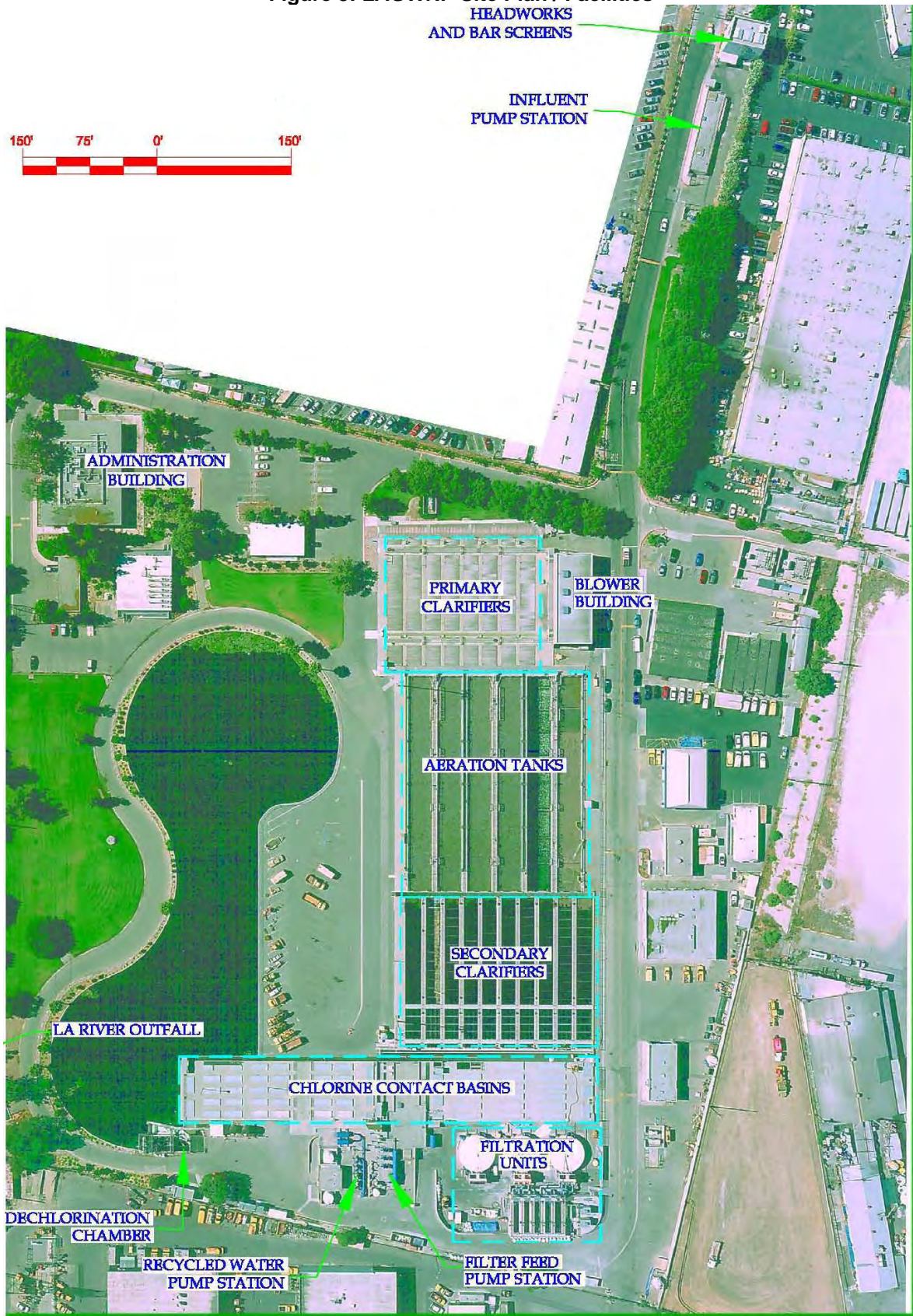
Figure 3: LAGWRP Site Plan / Facilities
